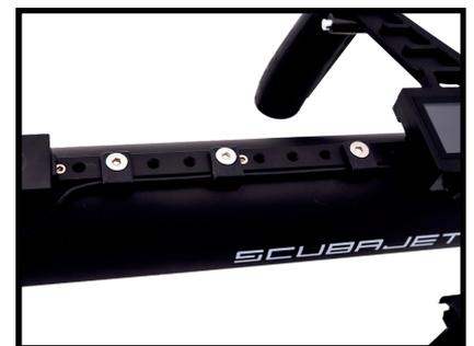
6. Secure the cable by creating a loop under the DHC and mounting it with cable clamps along the tube, maintaining consistent distances between the screws.
