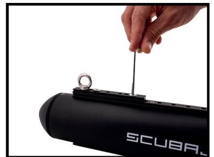
3. Position the short rail on top of the large rail on the tube, aligning the edges, and secure it with two screws using the larger Allen key.
