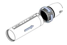
4 Attach the other tube and rotate it clockwise to secure and close it, then use the Allen key to reinstall the locking screw.
