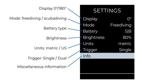
Navigate the menu using the left and right triggers on the Dual Hand Controller to adjust the settings. To confirm the changes, press one of the buttons.
