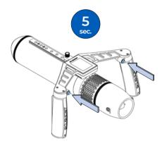
2 Turn the SCUBAJET on/off by pressing the 2 buttons on the Dual Hand Controller for 5 seconds.
