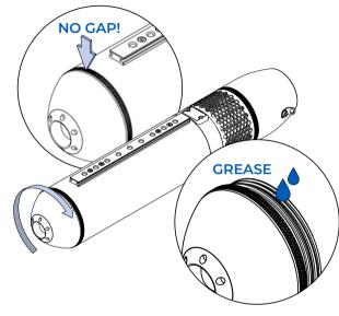
2 Make sure the grooves of the nose are well lubricated. Add some of the grease included if the nose is too hard to screw onto the tube. Ensure there's no gap between the tube and the nose, or water could get inside your SCUBAJET and cause damage. The nose and tube markers should align, indicating the nose is locked correctly. Your SCUBAJET might not turn on otherwise.
