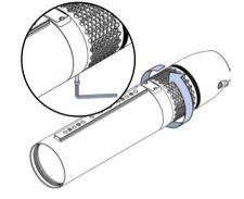
**3** Using an Allen key, remove the locking screw, then unscrew the motor unit counter-clockwise to remove the tube.
