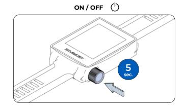
1 To turn on/off the remote control, press the button for 5 seconds.
