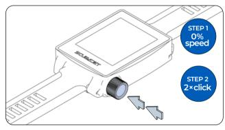
**3** To enter or exit the menu, set the speed to 0% first, then double-click on the wheel button. Toggle up and down the menu items by turning the wheel and confirm your selection by pressing it once.
