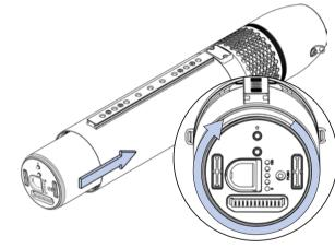
The battery has to be fully charged. Insert the battery and rotate the ring clockwise until the battery locks in place. Push the battery in until you hear a click; otherwise, the nose will not fit on the tube.
