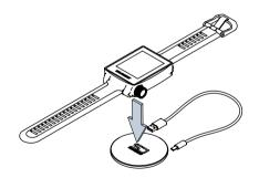
Place the remote in the middle of the charger until the light changes from red to blue. The remote begins charging only when the light turns blue. The display will show you when the remote is fully charged.
