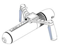
4 Press both triggers on the Dual Hand Controller to start your SCUBAJET. Set your speed to at least 4%. The default start setting is "Trigger Dual", which allows you to turn off the engine with just one trigger. You can always adjust the settings to customize your experience.
